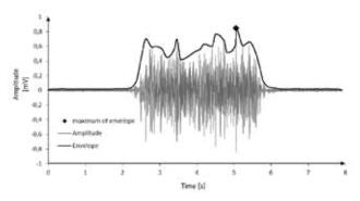
Figure 4. Exemplary envelope of an EMG signal
